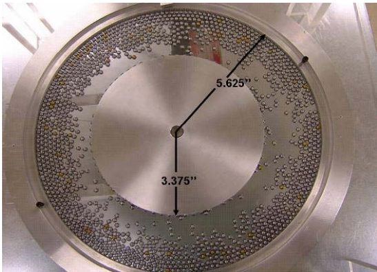
(Color online) Figure 2: Top view of the granular Shear Cell (GSC). Gravity acts into the page.
